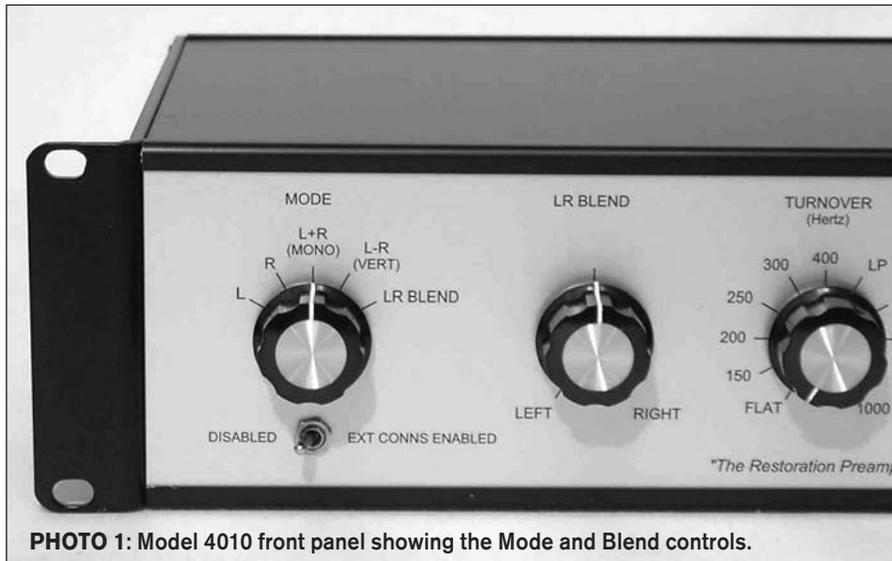
PHOTO 1: Model 4010 front panel showing the Mode and Blend controls.
