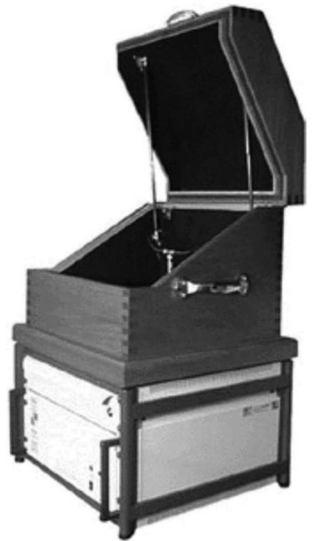
PHOTO 2: Microphone Calibration Workstation, model 9350C from the Modal Shop, Inc., [www.modalshop.com](http://www.modalshop.com). When the lid is closed, some sound isolation is provided for the microphone calibration.
