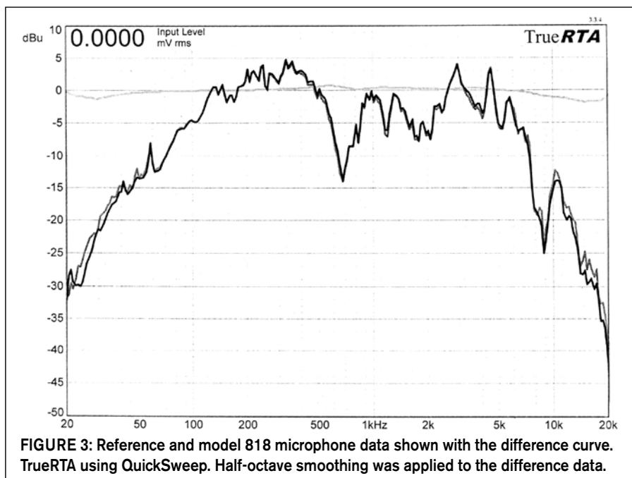
FIGURE 3: Reference and model 818 microphone data shown with the difference curve. *TrueRTA* using QuickSweep. Half-octave smoothing was applied to the difference data.
