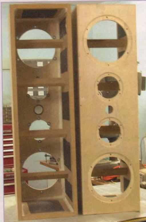
Photo 4: This will be a stereo pair of three-way speakers. The three inputs will be: base, midrange, and upper frequencies, once Ron completes the project.
